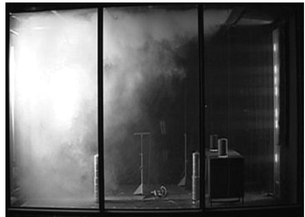
Room air flow visualization possible in the LTG lab (LTG Engineering Services)
