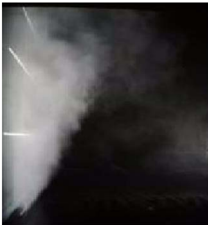
Picture 1a: Visualization of indoor air flow, start, 70 m 3 /h and -4 K
